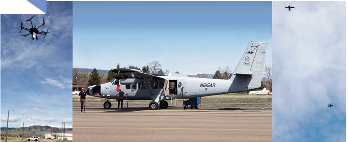
Figure 1. Left, Headwall turnkey UAV package with Co-Aligned VNIR-SWIR sensor and LiDAR flies a pre-programmed route in the Colorado sky, Center, National Science Foundation (NSF) Airborne Observation Platform (AOP) Twin Otter manned aircraft containing NASA-JPL AVIRIS-NG sensor prepares for takeoff on a nearby runway. Right, both aircraft flying above the same target area at the same time, but at very different altitudes.
