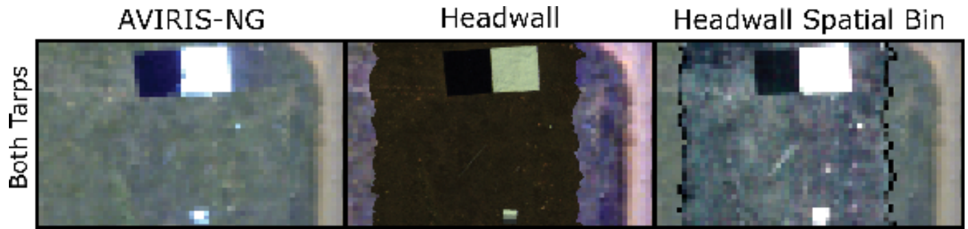
Figure 3. Left to right: AVIRIS-NG image of its reflectance calibration tarp, Headwall image of its tarp, and Headwall image resolution-matched.
