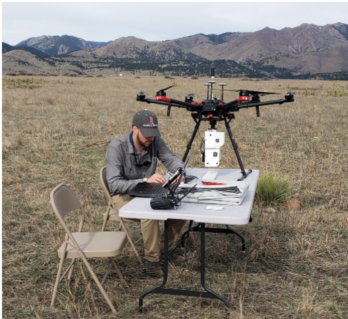
Figure 8. Photograph of the Headwall lightweight hyperspectral UAV platform being prepared for flight. The total take-off weight (TOW) of the platform including the hyperspectral payload is well within US Federal Aviation Administration (FAA) regulations on commercial drone piloting under Part 107 guidelines, and a large support team is not needed.
